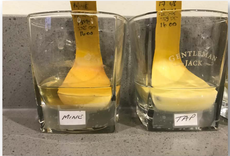
Swelling waterstop being tested with shaft waters VS tap water.
