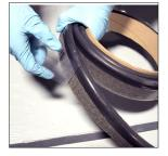
• Peel back the packing tape and release liner at the beginning of the reel.
