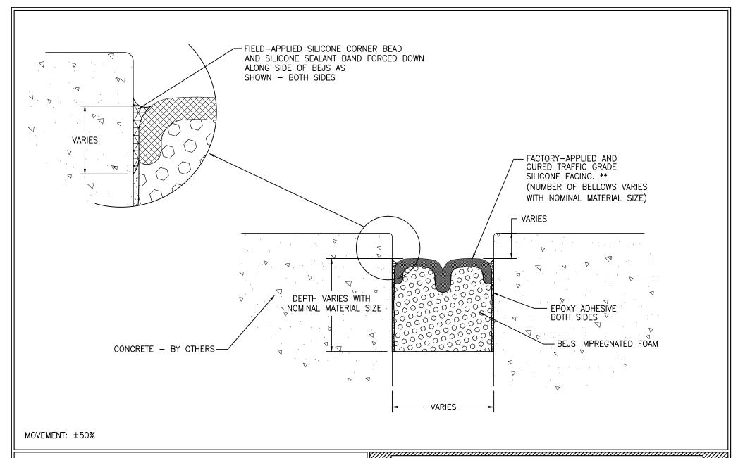
\*\* WIDTHS UNDER 1 1/4 -INCH (25mm) HAVE A CONVEX SINGLE-BELLOWS SURFACE. WIDTHS FROM 1 1/2 -INCH (25mm) TO 4-INCHES (100mm) HAVE A DUAL-BELLOWS SURFACE.
